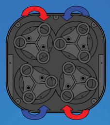
Opposite rotating heads mean the operator does NOT fight the machine.
